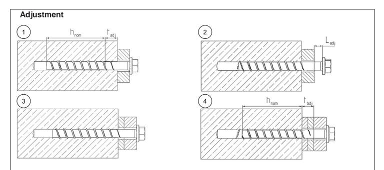
It is permissible to untighten the screw up to two times for adjustment purposes. Therefore the screw may be untightened to a maximum of  $L_{adj} = 20$  mm to the surface of the initial fixture. The total permissible thickness of shims added during the adjustment process is  $t_{adj} = 10$  mm.
