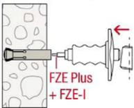
4.: Insert the anchor into the drill hole and then drive the expansion sleeve in with hammer-set device FZE Plus, using a manual hammer.
