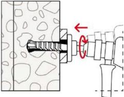
2.: Once the FZUB depth stop meets the fixture, create the drill hole undercut by making circular swiveling movements with the hammer drill while the hammer mechanism is engaged. Press the hammer drill firmly against the anchor base: 1 - 2 swiveling movements are sufficient for  $\varnothing$  14 mm, with 3 - 5 movements for  $\varnothing$  18 mm and  $\varnothing$  22 mm.
