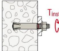
6.: Mount installation object (e.g. anchor plate), washer and nut, screw (for FZA I) or threaded rod with washer and nut (for FZA I) and apply installation torque with torque spanner.
