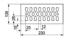
Lightweight aggregate concrete hollow block Hbl, EN 771-3:2015; e.g. Sepa according to Annex C 14
