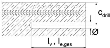
Measure and control concrete cover  $c$
