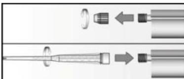
Twist off the sealing cap
