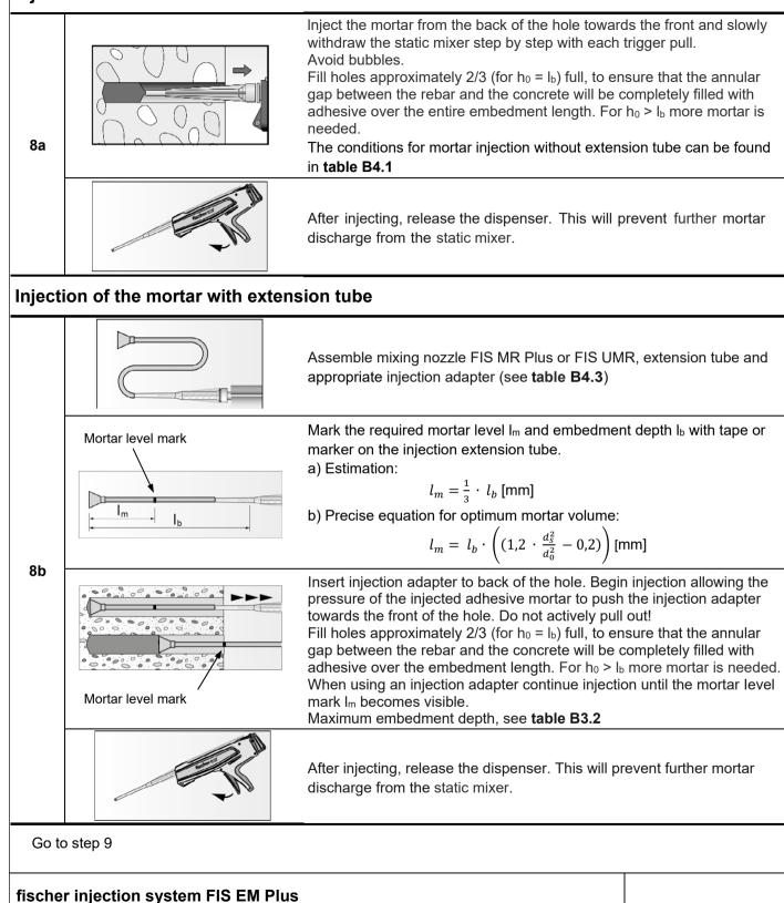
Intended Use Installation instruction part 4, mortar injection Annex B 8
