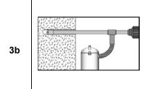
Use a suitable dust extraction system, e.g. fischer FVC 35 M or a comparable dust extraction system with equivalent performance data.
