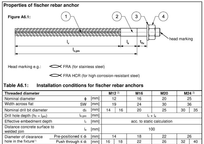
Minimum thickness of<br/>concrete member $h_{min}$ [mm] $h_0+30$ <br/>( $\geq 100$ ) $h_0+2d_0$ Maximum torque moment for<br/>attachment of the fixturemax T<sub>fix</sub>[Nm]50100150150
