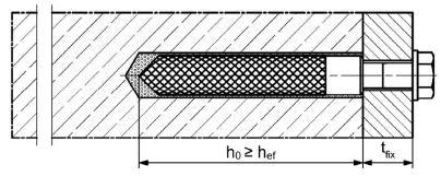
Pre-positioned installation with subsequently injected fischer filling disc (annular gap filled with mortar)
