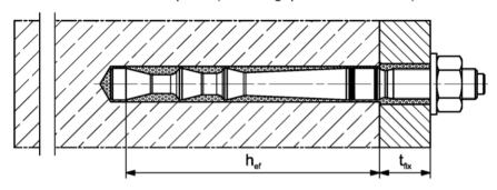
Pre-positioned or push through installation with subsequently pressed filling disk (annular gap filled with mortar)
