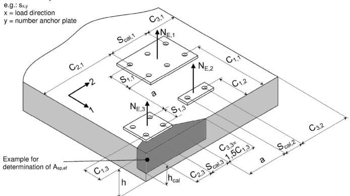
Example for different anchor plates: For considering all free edges the direction 1 and 2 must be swaped.
