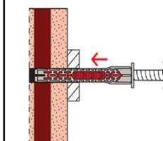
3. Insert anchor (screw and sleeve) by using a hammer until the collar of the plastic sleeve is flush with the surface of the fixture.
