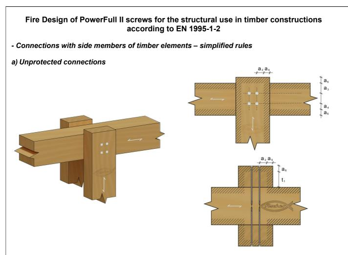
Figure N1.1: Fire design for unprotected screws – laterally loaded (figures not to scale)
