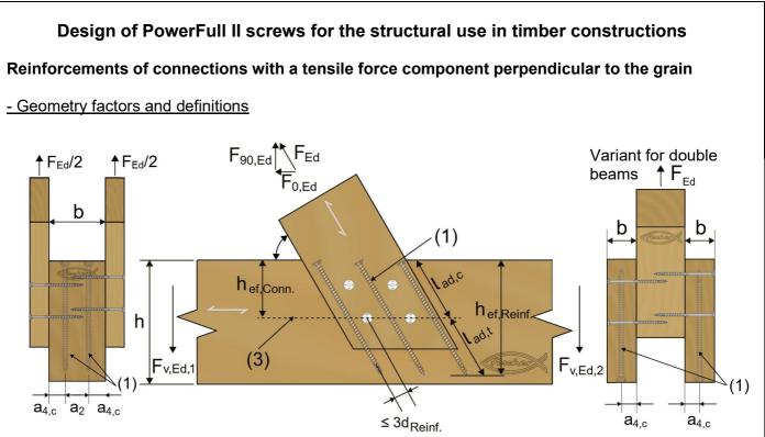
Figure K1.1: Joint with a tensile force component – reinforcement with internal screws (figures not to scale)
