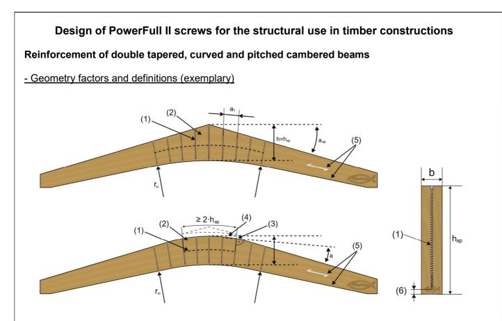
Figure G1.1: Internal reinforcement of beams with screws (figures not to scale)
