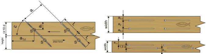
Figure E1.1: Mechanically jointed beams with inclined screws (figures not to scale)
