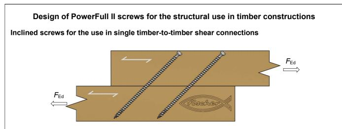
Figure M2.1: Shear connection with inclined screws timber-to-timber connection (figure not to scale)
