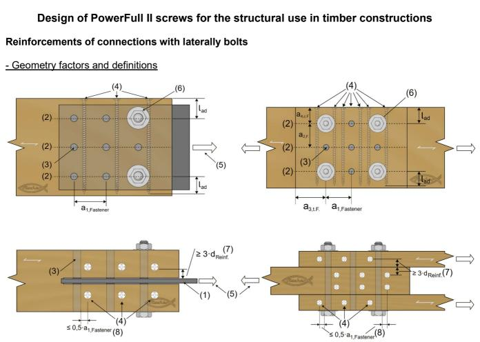
Figure J1.1: Shear connections with bolts – reinforcements with internal screws (figures not to scale)
