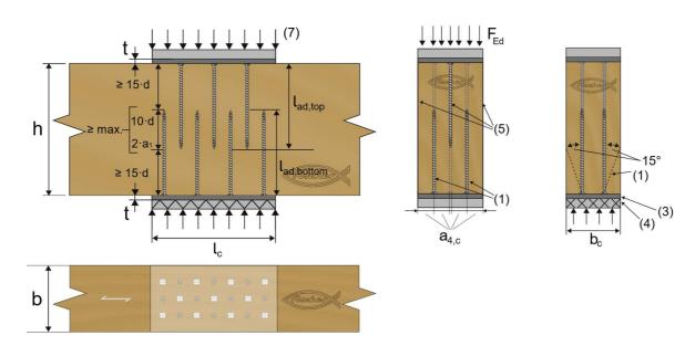
Figure F2.1: Reinforcement to transfer loads perpendicular to the grain-direction (figures not to scale)
