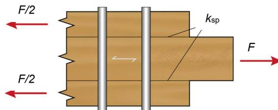
Figure D16.1: Definition of the shear plane  $k_{sp}$  (figure not to scale)
