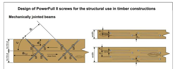
Figure E2.1: Mechanically jointed beam with crossing screws (figures not to scale)
