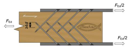
Figure M1.1: Shear connection with inclined screws steel-to-timber connection (figure not to scale)
