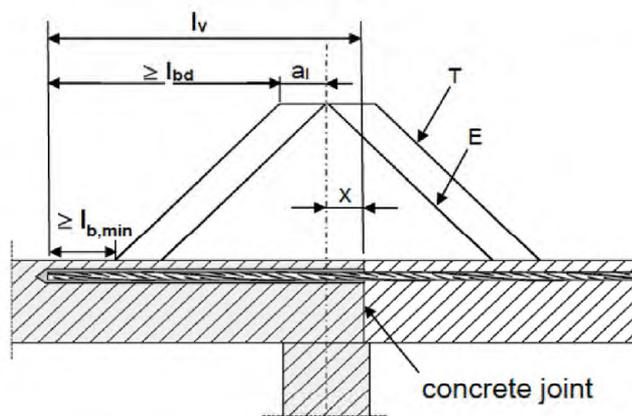
(only post-installed rebar is plotted)
