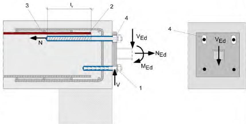
The required transverse reinforcement acc. to EN 1992-1-1:2004+AC:2010 is not shown in the figures. **The fischer rebar anchor FRA may be only used for axial tensile force.** The tensile force must be transferred by lap to the existing reinforcement of the building. The transfer of the shear force has to be ensured by suitable measure, e.g. by means of shear force or anchors with European Technical Assessment (ETA)
