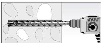
Drill the hole to the required embedment depth using a hammer drill with carbide drill bit set in rotation hammer mode or a pneumatic drill.
