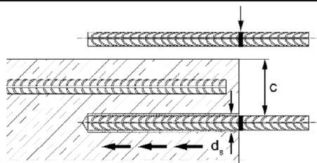
Before use, make sure that the rebar or the fischer rebar anchor is dry and free of oil or other residue.
