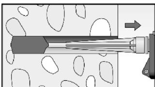
Inject the mortar from the back of the hole towards the front and slowly withdraw the mixing nozzle step by step with each trigger pull. Avoid bubbles.
