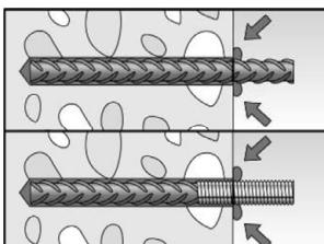
After installing the rebar or fischer rebar anchor the annular gap must be completely filled with mortar.
