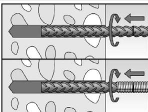
Insert the rebar / fischer rebar anchor slowly twisted into the borehole until the embedment mark is reached.
