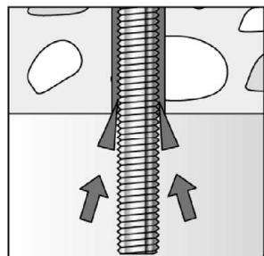
For overhead installation, support the rebar / fischer rebar anchor and secure it from falling till mortar started to harden, e.g. using wedges.
