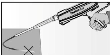
Press out approximately 10 cm of mortar until the resin is permanently grey in colour. Mortar which is not grey in colour will not cure and must be disposed.
