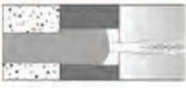
For push through installation (not FIS E) fill the annular gap also with mortar.           |
