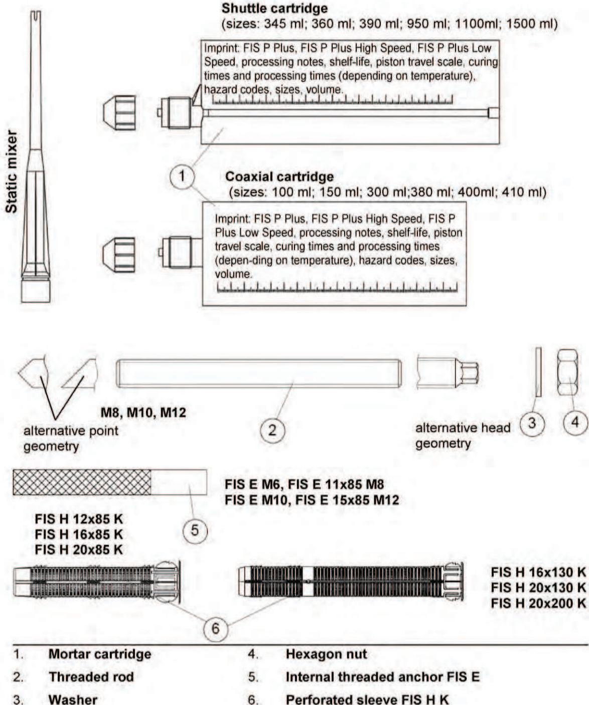
fischer Injectionsystem FIS P Plus for masonry
