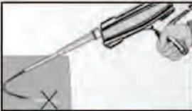
Press out approximately 10 cm of material until the mortar is permanently grey in colour. Mortar which is not grey in colour will not cure and must be disposed off.         |
