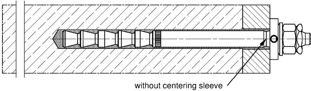
Push through installation without shear force sleeve, FHB dyn (annular gap filled with mortar)
