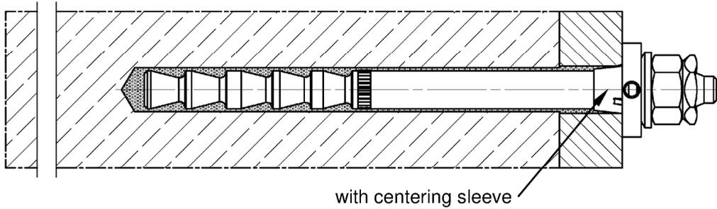
Push through installation with shear force sleeve, FHB dyn V (annular gap filled with mortar)
