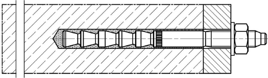
**Pre-positioned or push through installation with subsequently injected fischer filling disc**
