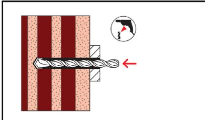
1. Drill the bore hole as per Table B2.1 using the drilling method described in the corresponding Annex C.
