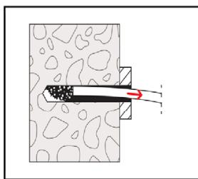
For application in hollow or perforated bricks, removal of bore dust is not necessary.
