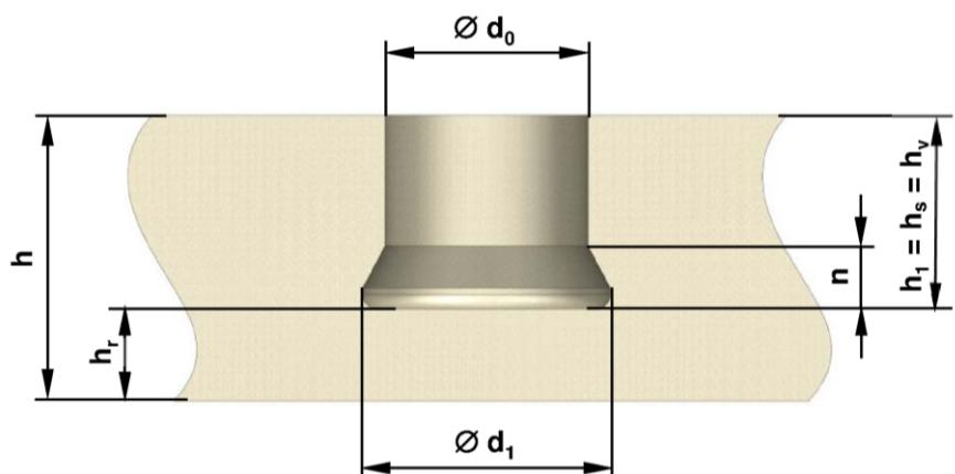
**Figure B3: Geometrie of drill hole**
