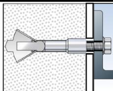
5b: If the anchor cannot support against the fixture (with cover layer) no installation torque may be applied ( $T_{\max} = 0$ )
