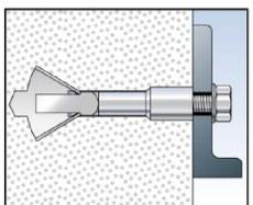
5a: Optional tightening the fastener with a torque  $T_{\max} \leq 3 \text{ Nm}$ . The anchor could be pulled against the fixture depending on the compressive strength of the AAC.
