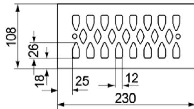
Lightweight aggregate concrete hollow block Hbl, EN 771-3:2015; e.g. Sepa according to Annex C 14
