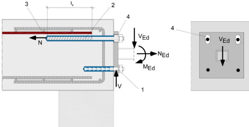
The required transverse reinforcement acc. to EN 1992-1-1:2004+AC:2010 is not shown in the figures. **The fischer rebar anchor may be only used for axial tensile force.** The tensile force must be transferred by lap to the existing reinforcement of the building. The transfer of the shear force has to be ensured by suitable measures, e.g. by means of shear force or anchors with European Technical Assessment (ETA).
