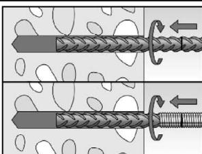
Insert the rebar / fischer rebar anchor slowly twisted into the borehole until the embedment mark is reached.
