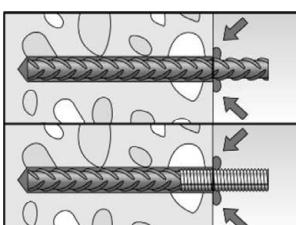
After installing the rebar or fischer rebar anchor the annular gap must be completely filled with mortar.
