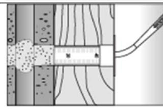
Fill the sleeve with mortar beginning from the bottom of the drill hole. <sup>1)</sup> For deep drill holes use an extension tube. |
