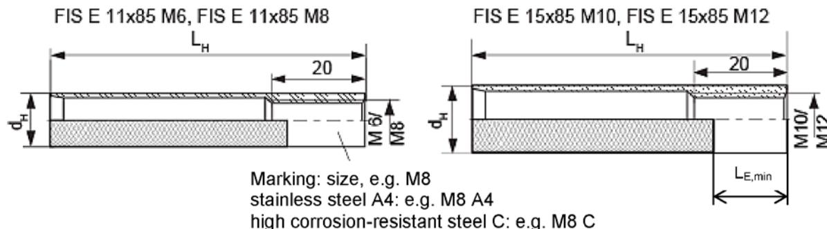
**Table B1.2: Installation parameters (internal threaded anchor FIS E without perforated sleeve)**
