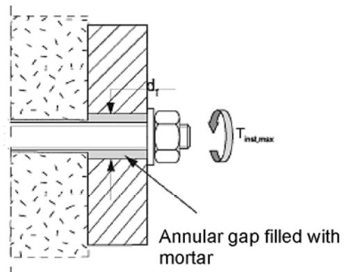
Internal threaded anchors FIS E without perforated sleeve FIS H K; Installation in solid brick masonry and aerated concrete
