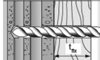
Drill the hole through the fixture. Depth of drill hole ( $h_0+t_{fix}$ ) and drill hole diameter see Table B1.4                     |
