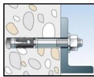
5: Installed fastener
