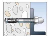
7: Installed fastener
