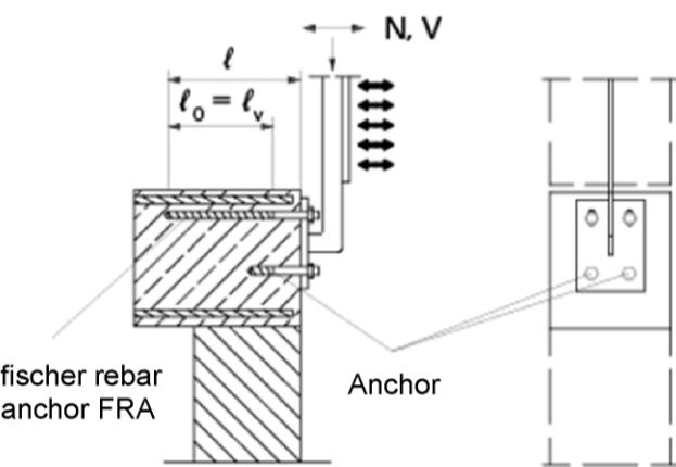
**Figure A7:** Lap of the anchoring of guardrail posts.
