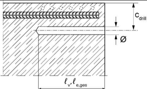
Measure and control concrete cover  $c$
