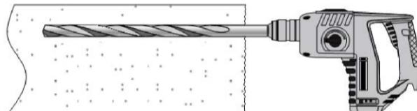
Drill hole to the required embedment depth using a hammer-drill with carbide drill bit set in rotation hammer mode or a compressed air drill.
