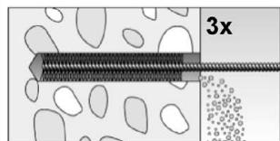
Brush drill hole three times; for drill hole diameters  $d_0 \geq 30 \text{ mm}$  attach brush to a power tool and brush hole with a speed of max. 550 revolutions per minute. For deep holes a brush extension is mandatory. Use suitable brushes (see Table B6.2).
