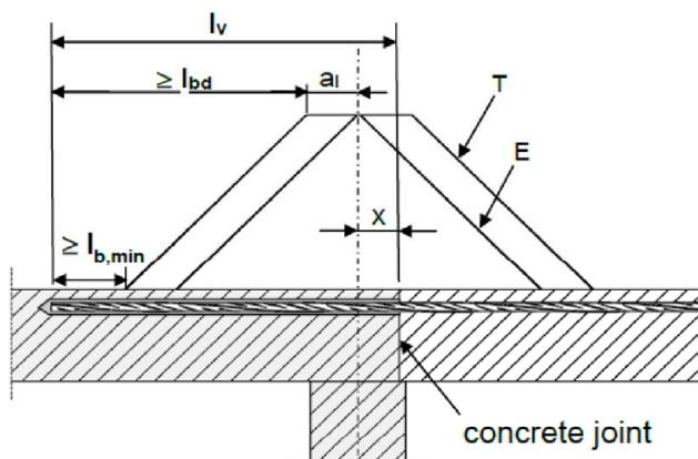
(only post-installed rebar is plotted)
