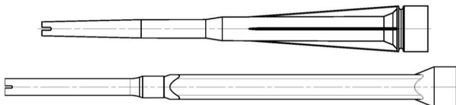
**Injection adapter and Extension tube for static mixer**
