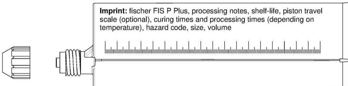
**Injection cartridge (coaxial cartridge) with sealing cap; Size: 100 ml, 150 ml, 300 ml, 380 ml, 400 ml, 410 ml**
