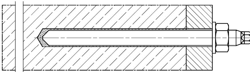
Pre-positioned installation with subsequently injected fischer filling disc (annular gap filled with mortar)
