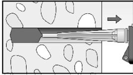
Inject the mortar from the back of the hole towards the front and slowly withdraw the mixing nozzle step by step after each trigger pull. Fill holes approximately 2/3 full, or as required to ensure that the annular gap between the rebar and the concrete is completely filled with adhesive over the embedment length.
