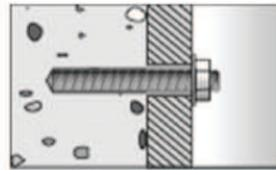
For push-through installation fill the annular gap also with mortar.
