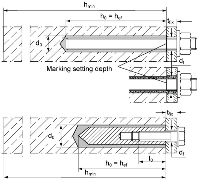
**Upat threaded rod** pre-positioned anchorage
