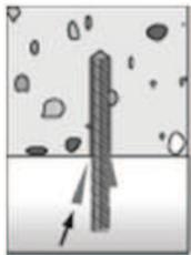
For overhead installation support the anchor element with wedges.
