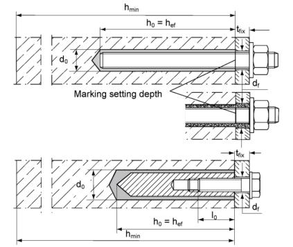
**Upat threaded rod** prepositioned anchorage
