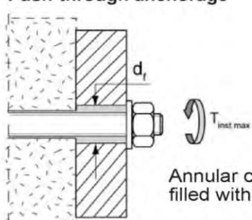
Internal threaded anchors UPM-I without perforated sleeve UPM SH K; installation in solid brick masonry and autoclaved aerated concrete
