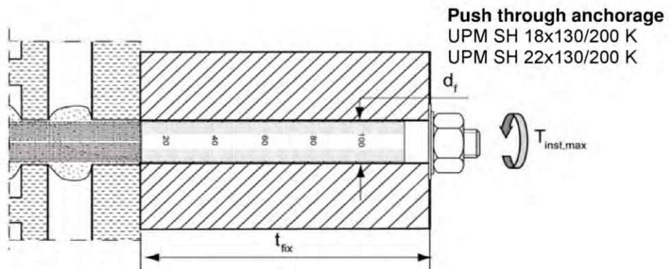
Internal threaded anchor UPM-I with perforated sleeve UPM SH K; Installation in perforated and solid brick masonry
