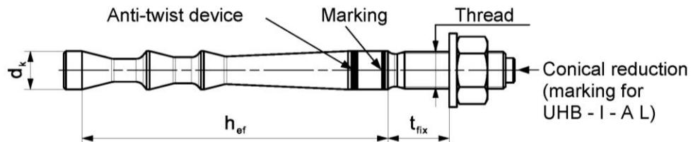
**Marking:** work symbol, size of anchor, setting depth. e.g.: UHB-I M10x95
