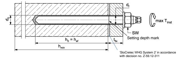
Fastening system 'fischer injection system FIS EM Plus' for use in coated concrete surfaces in SFH facilities
