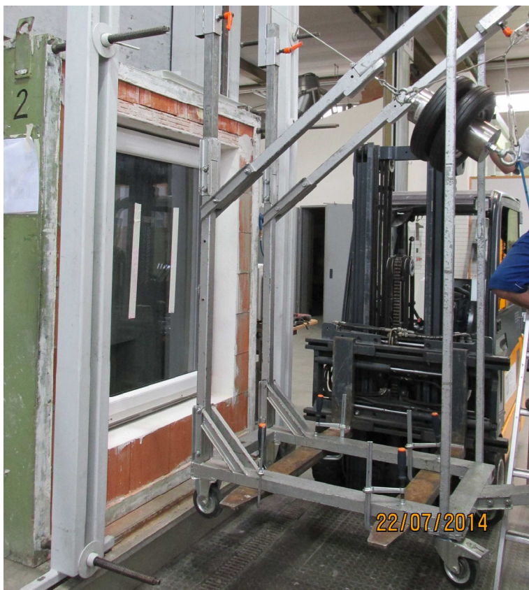
Fig. 16 Test setup pendulum impact
