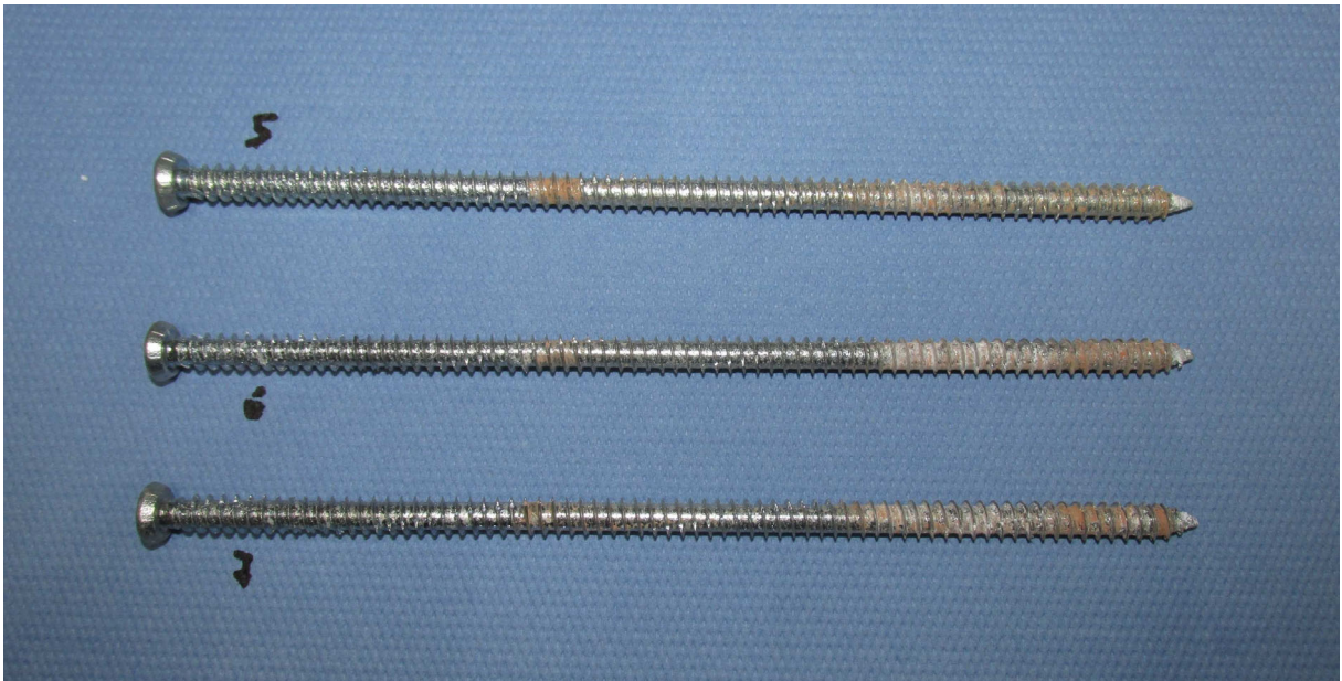
Fig. 20 Condition of the window frame screws FFS 7.5 x 202 with some slight deformations after dismantling
