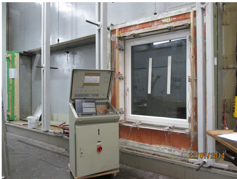
Fig. 9 View of test specimen with attached measuring points
